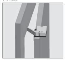
Clamped on the door with two brackets (screwed with 2 long screws and nuts).
