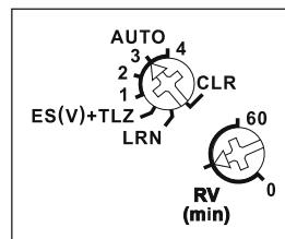
Switch on/off with wireless pushbutton. Switch on if motion is detected and optionally if brightness is insufficient. Switch off if no motion is detected by all FBHs and RV time elapses.
