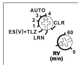
Switch on/off with wireless pushbutton. Switch on if motion is detected and brightness is insufficient. Switch off all FBHs and FAHs if no motion is detected and brightness is sufficient and RV time elapses.
