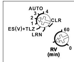
Switch on/off with wireless pushbutton, switch off if no motion is detected or brightness of all/one FBH or FAH is sufficient and RV time elapses.
