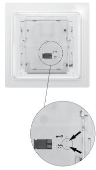
Insert the encryption plug and operate the rocker.
