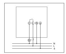
The device can be manually activated with a circuit breaker. After releasing the button (return of power) the device switches on (for at least 40 secs or for the time set on the device).
