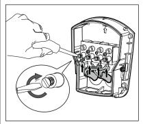
■ Connect the individual wires to the appropriate terminal.
