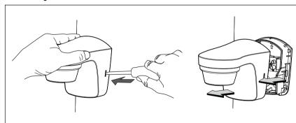
Using the screwdriver, carefully loosen the snap-in hook at the side and pull the device forward.
