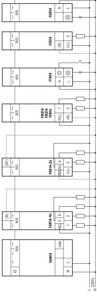
The attached second terminator should be plugged to the last actuator. or a terminating resistor has to be clamped to the terminals RSB/RSA of the last energy meter ( $120\,\Omega$ , not included).
