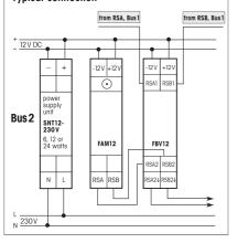
**Bus 1** signals are tapped by RSA/RSB and transmitted directly to the antenna module FAM12 in **Bus 2**.
