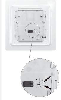
Insert the encryption plug and operate the rocker.
