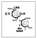
The minimum brightness (fully dimmed) is adjustable with the upper %♣ rotary switch. In the setting LRN up to 35 pushbuttons can be assigned, of which one or more central pushbuttons.
