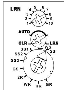
The upper and the middle rotary switches are for teaching-in the sensors. In normal mode, the middle rotary switch is then set to AUTO and the bottom rotary switch to the required function:
