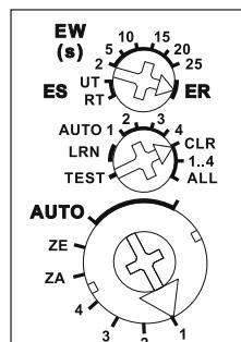
**The upper rotary switch** defines the function of the 4 channels together as impulse switch with universal switch (ES-UT), as impulse switch with direction switch (ES-RT), as fleeting NO contact (EW) or as relay (ER). In ES function, central control commands ON/OFF can be taught-in. In EW function, a wiping time of 2 to 25 seconds can be set.
