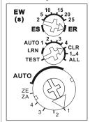
The upper rotary switch defines the function of the 4 channels together as impulse switch (ES). fleeting NO contact (EW) or relay (ER). In ES function, central control commands ON/OFF can be taught-in. In EW function, a wiping time of 2 to 25 seconds can be set.
