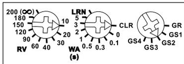
With the middle rotary switch on the side in the setting LRN up to 35 wireless pushbuttons can be assigned, of which one ore more central pushbuttons. Then the automatic turning system (WA) is set using the same rotary switch.
