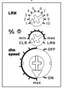
The minimum brightness (fully dimmed) is adjustable with the %♣ rotary switch. In the setting LRN up to 35 wireless pushbuttons can be assigned therefrom one ore more central pushbuttons.
