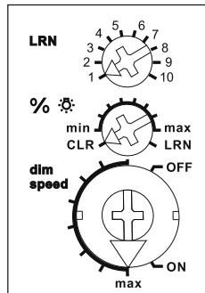
The minimum brightness (fully dimmed) is adjustable with the % rotary switch. In the setting LRN up to 35 wireless pushbuttons can be assigned therefrom one ore more central pushbutton.
