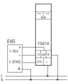
At more than 2 devices side by side, an half pitch must stay free for ventilation. Place the DS14 spacer on the right side and use the 1.5 pitch width jumper. For the control from several LED drivers with 1-10V passive interface, an additional voltage source is necessary, this can be the power supply unit SNT12-230V/12V DC-0.5A or SNT61-230V/12V DC-0.5A, in both cases a 1kOhm resistor is necessary.
