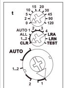
**Use the rotary switches** to teach-in the buttons and test the 2 channels as required. For normal mode, the middle and lower rotary switches are then set to AUTO. With the upper rotary switch the EW time (0-120 seconds) is directly set for relays or the RV time (0-120 minutes) for impulse switches for all channels if necessary.
