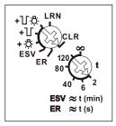
With the top rotary switch in the setting LRN up to 35 wireless pushbuttons can be assigned therefrom one ore more central control pushbuttons. In addition wireless window/door contacts with the function N/O contact or N/C contact while the window is open, wireless outdoor brightness sensors FAH and wireless motion/brightness sensors FBH. The required function of the impulse switch with integrated relay function can then be selected:
