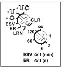
With the top rotary switch in the setting LRN up to 35 wireless pushbuttons can be assigned, of which one or more central control pushbuttons. In addition wireless window/door contacts with the function N/O contact or N/C contact while the window is open. The required function of the impulse switch with integrated relay function can then be selected:
