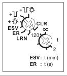
With the top rotary switch in the setting LRN up to 35 wireless pushbuttons can be assigned therefrom one ore more central control pushbuttons. In addition wireless window/door contacts with the function N/O contact or N/C contact while the window is open. The required function of the impulse switch with integrated relay function can then
