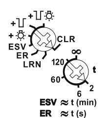
**With the top rotary switch** in the setting LRN up to 35 wireless pushbuttons can be assigned thereto from one or more central control pushbuttons. In addition wireless window/door contacts with the function N/O contact or N/C contact while the window is open, wireless outdoor brightness sensors FAH and wireless motion/brightness sensors FBH. The required function of the impulse switch with integrated relay function can then be selected:
