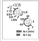
With the top rotary switch in the setting LRN up to 35 wireless pushbuttons can be assigned therefrom one or more central control pushbuttons. In addition wireless window/door contacts with the function N/O contact or N/C contact while the window is open, wireless outdoor brightness sensors FAH and wireless motion/brightness sensors FBH. The required function of the impulse switch with integrated relay function can then be selected:
