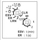
With the top rotary switch in the setting LRN up to 35 wireless pushbuttons can be assigned therefrom one ore more central control pushbuttons. In addition wireless window/door contacts with the function N/O contact or N/C conatct while the window is open. The required function of the impulse switch with integrated relay function can then be selected:
