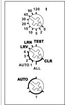
**Use the rotary switches** to teach-in the pushbuttons and test the device as required. For normal mode, the middle and lower rotary switches are then set to AUTO. With the upper rotary switch the EW time (0-120 seconds) is directly set for relays or the RV time (0-120 minutes) for impulse switches for all channels if necessary.
