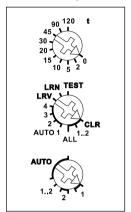
**Use the rotary switches** to teach-in the pushbuttons and test the 2 channels as required. For normal mode, the middle and lower rotary switches are then set to AUTO. With the upper rotary switch the EW time (0-120 seconds) is directly set for relays or the RV time (0-120 minutes) for impulse switches for all channels if necessary.
