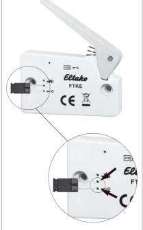
Insert the encryption plug and pull the lever.
