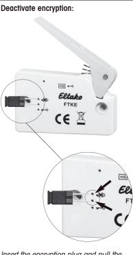
Insert the encryption plug and pull the lever.
