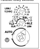
The upper rotary switch LRN is required for teach-in. Then the off-delay 1 to 30 minutes can be set.
