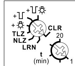
With the top rotary switch in the setting LRN up to 35 wireless pushbuttons and/or wireless motion/brightness sensors FBH can be assigned of which one ore more central pushbuttons. The required function of this staircase off-delay timer can then be selected:
