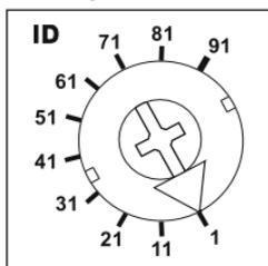
The rotary switch assigns a separate ID range to a maximum of 10 FTS12EM's.
