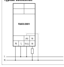
Rated switching capacity 10A/250V AC Incandescent lamp and halogen lamp load 1) 230V
