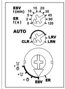
The function of the actuator is set with the lower rotary switch.
