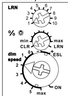
**The minimum brightness (fully dimmed) is adjustable with the % rotary switch.**
