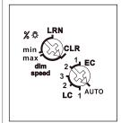
The minimum brightness (fully dimmed) or the dimming speed is adjustable with the upper %-\$/dimming speed rotary switch.
