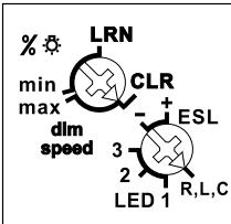
The minimum brightness (fully dimmed) or the dimming speed is adjustable with the %/dimming speed rotary switch. In the setting LRN up to 35 wireless pushbuttons can be assigned, of which one or more central pushbuttons.
