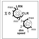
The minimum brightness (fully dimmed) is adjustable with the %# rotary switch. In the setting LRN up to 35 wireless pushbuttons can be assigned therefrom one or more central pushbuttons.
