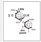
The minimum brightness (fully dimmed) is adjustable with the %☆ rotary switch. In the setting LRN up to 35 wireless pushbuttons can be assigned therefrom one or more central pushbuttons.
