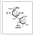
The minimum brightness (fully dimmed) is adjustable with the %. Totary switch. In the setting LRN up to 35 wireless pushbuttons can be assigned therefrom one or more central pushbuttons.
