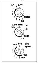
The upper rotary switch determines the operation, whether automatic lamp detection or special comfort positions should work:
