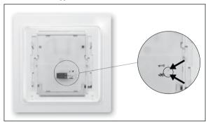
Insert the encryption plug and operate the rocker.
