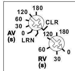
The upper rotary switch AV is required for teach-in. Then set here the response lag time AV between 0 and 180 seconds for Contact L-2.
