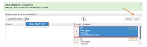
figure 21: add sensor/actuator
